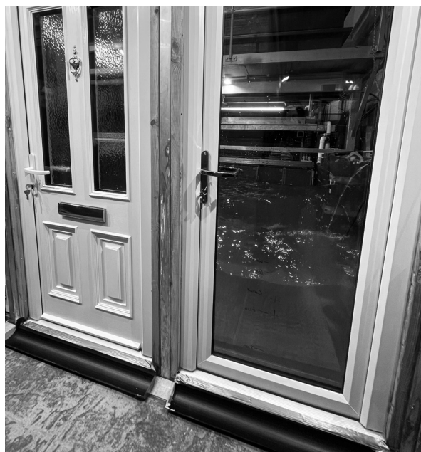
Composite & UPVC doors shown in BSI approved test facility undergoing test
