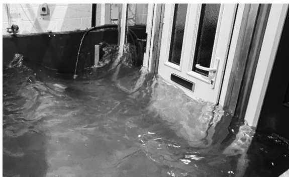
Composite & UPVC doors shown during wave test
